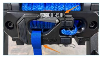
**22.** Tie a knot in the retractor cable approximately 2 inches from the end. Ensure the rubber washer is positioned as shown. Attach the split ring to the winch remote and place the remote in the holder.
