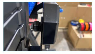
21. Attach the hook to the winch rope and secure to the fairlead with the provided cable ties. Trim the loose ends.
