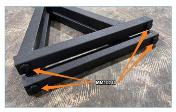
2. Fasten the lower tube assembly to the right frame through the inside of the tube as shown using an M8x25mm hex flange bolt and M8 fender washer. Repeat for the other side and left frame. Leave these hand-tight for now.
