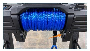
19. Fasten the winch to the frame with the (4x) M10x60mm bolts, lock washers, flat washers and the square nuts provided with the winch (6mm Allen key).
