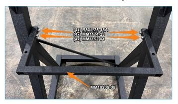
6. Rotate the leveling feet until each side of the frame is level front to back then, adjust the center mount until it's level and tighten the (4x) bolts from the previous step (5mm hex key). Now fully tighten the (2x) bolts from step 2 (13mm wrench) and the (2x) bolts from step 4 (5mm hex key).
