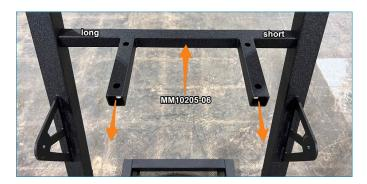
4. Install the brace between the left and right frames using (2x) M8x25mm button head bolts, lock washers, and flat washers. Leave hand-tight for now.
