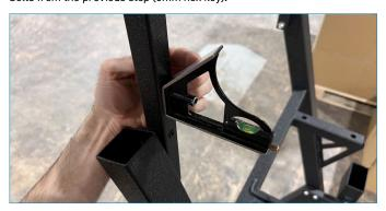
10. Fasten the retractor to bracket 3 as shown using the (2x) M4x6mm button head bolts. Tighten using a 3mm hex key.
