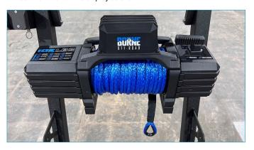
17. Lift up one side of the winch and slide one of the fairlead brackets under the mounts.
