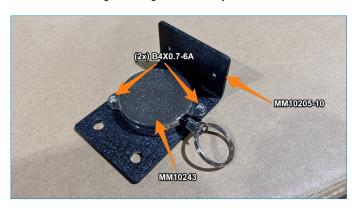
11. Fasten the remote holder to bracket 3 as shown using (2x) M4x6mm flat head bolts, washers, lock washers, and hex nuts. Tighten using a 3mm hex key and 7mm wrench.
