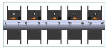
24. Install the rope spool and tube assembly into the frame using (2x) M8x45mm button head bolts, lock washers, and flat washers (5mm Allen key). Rotate the tube so the M4 bolts from the previous step are facing to the rear and down so they are hidden.
