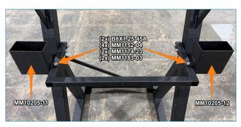
8. Install the (2x) upper mounts to the left and right frames using (4x) M8x45mm button head bolts, lock washers, and flat washers. Ensure the rivet nuts in the upper mounts are facing forward. Leave hand-tight for now.
