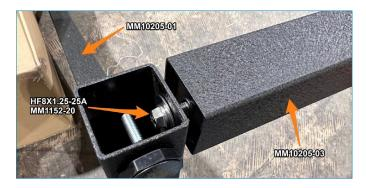
3. Stand the frame up in its normal position. Install the upper mount into the square holes in the left and right frames ensuring the orientation of the "long" and "short" sides are as shown, and the mounts are facing forward.
